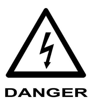
Dangerous voltage may exist for 3 minutes after removing power
